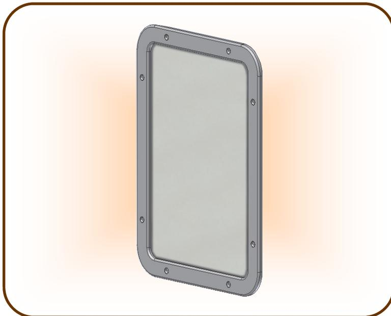
**JCP Specifications:** The overall size of the large mirror assembly is 12-3/8" x 16-3/8" x 5/16" thick, with the actual mirror area of 10" x 14". The mirror panel is 20 gauge stainless steel polished to a mirror finish approximating that of glass. The mirror frame is 14 gauge steel with a satin chrome finish.
